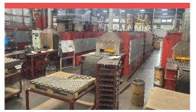
Continuous Sintering Furnaces ranging from 14 inches – 24 inches; we also offer multiple treatments and platings.
