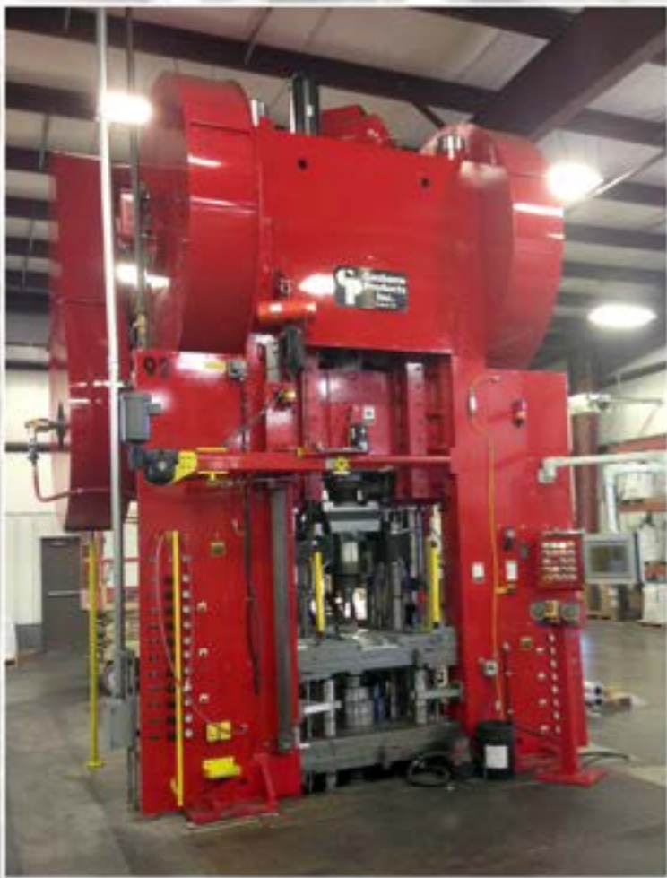
Gasbarre 750 Ton Powder Metal Press located at Sintergy's Reynoldsville, PA production facility.
